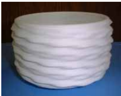
Fig.12 Nylon teabowl with 5% fluctuations and 3 orbits
