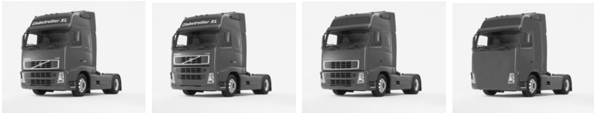
Fig. 3. Three examples of syntactic variations implemented for establishing visual effect of design elements. Far left: original appearance. Alterations from left to right: set of grilles repositioned; logotypes and emblems removed; shut lines, body lines, and set of grilles removed.
