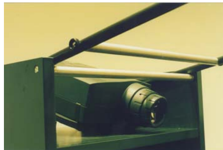
Figure 10: It may be necessary to rotate the excentered, horizontal rod, situated up front in the rack.
