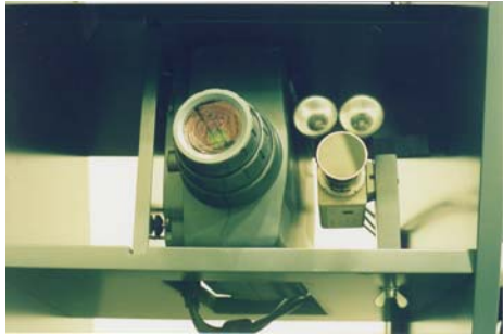
Figure 8: Slide the second beamer into the rack from the front side of the rack (left) and cable it. This is called the above view beamer. Fix and cable the video and lamps. Adjust the lateral positioner (right) of the above view beamer. Turn on the system switch in the bottom of the rack.
