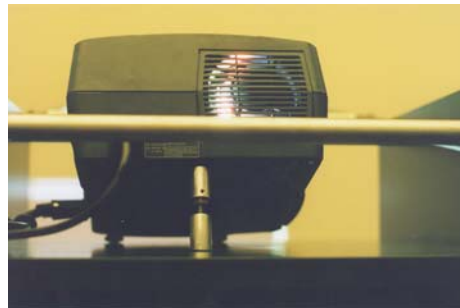
Figure 6: Position and cable one beamer at the top level of the rack. This is called the side view beamer. Adjust the vertical screw of the side view beamer
