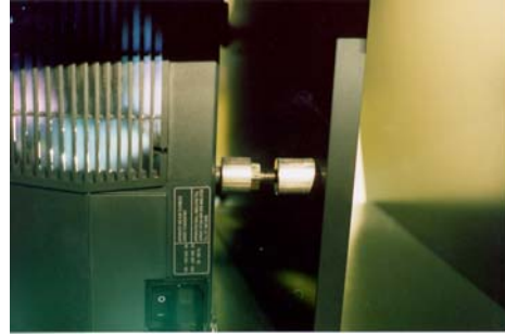
Figure 8: Slide the second beamer into the rack from the front side of the rack (left) and cable it. This is called the above view beamer. Fix and cable the video and lamps. Adjust the lateral positioner (right) of the above view beamer. Turn on the system switch in the bottom of the rack.
