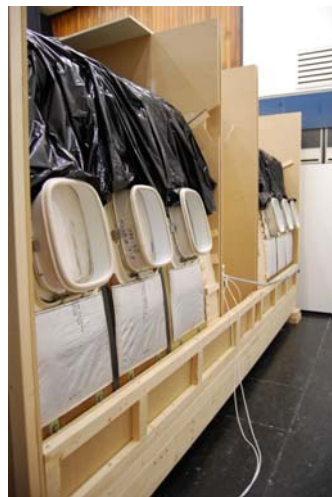
Figure 11: External view of aircraft cabin simulator
