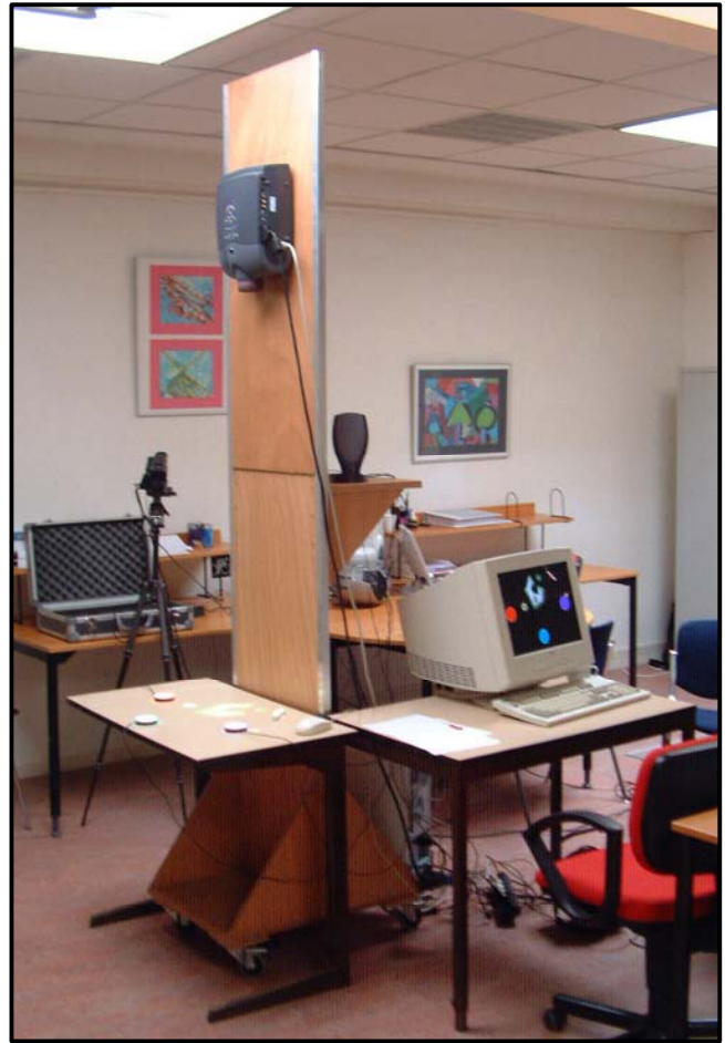
Figure 3. The set-up in the development environment, with the mount for the projector and the tabletop user interface. The graphics displayed in the programmer's monitor to the right are projected on the table to the left for the players.
