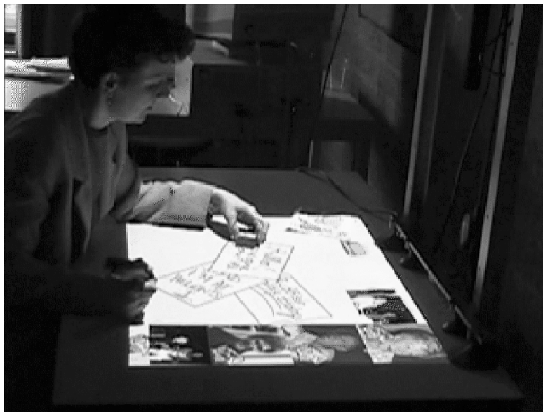
Figure 2 : Electronic notes are moved, rotated and stacked in a manner similar to paper notes.
