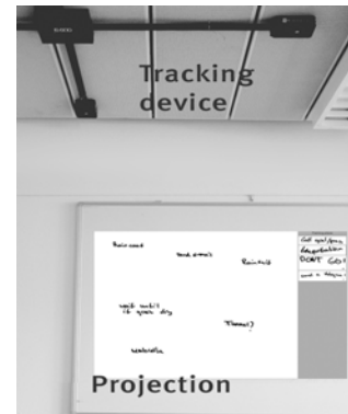
Figure 2: Attached to the roof is the device that tracks the SoniDisc, the ideas are shown with a projector.
