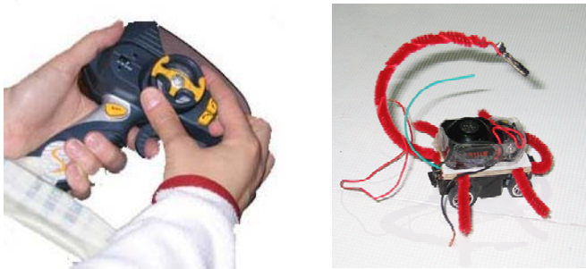
Figure 2. (Left) The adapted Pistol controller with a GamePad input device wired at its base. (Right) Close up picture of the Scorpion cars showing the wires used for balancing, the cable for battery charging, the wire-antenna for remote control. On top of the vehicle is mounted a ‘sonic disk’ for tracking through the ISense 600 system.
