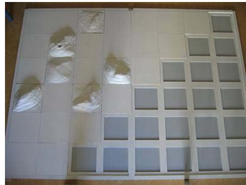
Figure 3: The physical part of the Active Landscape Grid is a hardboard grid on which cardboard tiles are fitted. Tiles can be flat or can have a relief upon them to provide a 3D morphology for the landscape.
